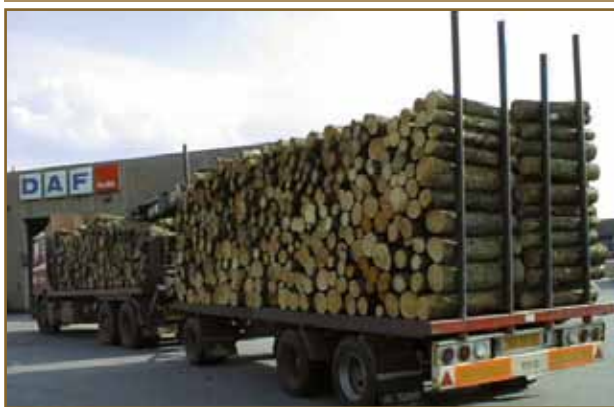
Fig. 69. Timber stacked transversely is not recommended!
