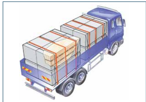
Fig. 51. Secured full load of sawn timber
